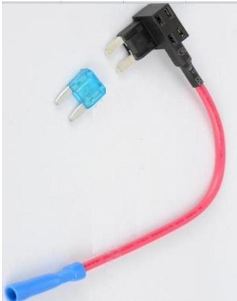
The item in the picture is a piggy back plug for the mini fuse slots. You simply install your original fuse (if there was one) in the bottom slot, and the desired fuse in the top slot, and plug it into the fuse box in place of your original fuse. This puts your original fuse back in circuit, and also provides you a short fly lead that you can attach your required relay to for a key controlled circuit.
